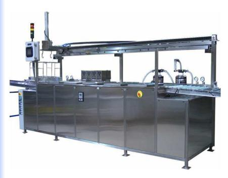
Zenith's TRANSTAR Automation System, one of 4 different automation designs available, is an overhead pick & place robotic system which completely automates a multi-stage ultrasonic cleaning or passivation process by transferring baskets of parts through the entire process fully automatically without the need for operator handling. This system provides for complete process repeatability and is fully user-programmable to adjust the system to suit any cleaning application.
