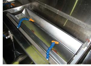
After exiting the ultrasonic cleaning reactor, compressed air knives gently remove over 90% of the detergent from the wire to prevent the detergent from entering the rinsewater. This feature greatly extends the life of the rinse water thereby further reducing water consumption.
