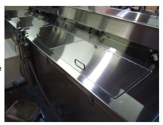
The wire then enters the Ultrasonic Rinse Reactor, where all remaining detergents are removed ultrasonically. User-adjustable spray assemblies are included to enhance the rinsing action.
