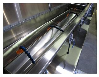
The SSW-132 is positioned at the exit side of the drawing equipment. wire is fed through the system using existing pay-out and take-up equipment. If such equipment does not exist, Zenith can provide it as well.
