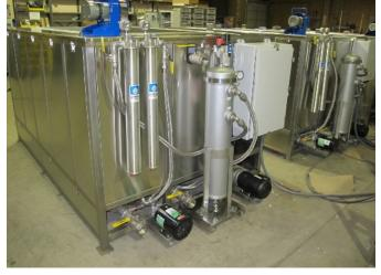
while simultaneously sweeping the surface of the fluid to remove any floating contaminants which could re-deposit onto the parts when they are removed from the tank.
