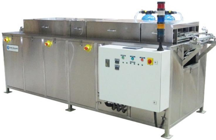
The ORBIT continuous conveyor ultrasonic cleaning system is very similar to a spray washing system where parts are placed onto a moving conveyor belt to be cleaned, rinsed, and dried as the parts pass through the system. The difference is that with the ORBIT, ultrasonic systems are used to do the cleaning rather than spray nozzles. As a result, parts are cleaned more thoroughly and completely.
