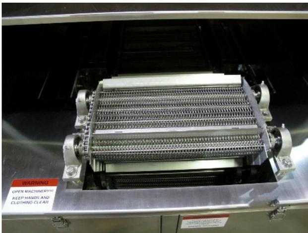
Parts are placed onto the conveyor belt or custom fixtures that Zenith can provide to support the parts being cleaned. This belt either moves continuously or intermittently using external signals from existing robotic part loading systems. The parts are first moved through the included CROSSFIRE Multiple Frequency Ultrasonic System which removes the contaminants. The cleaning chamber is continuously filtered while floating particles are swept from the surface .
