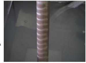
By oscillating the product intermittently, items being cleaned are scanned through the standing waves, thereby producing a more even scrubbing effect on the parts in the same way that a turntable in a microwave oven heats food more evenly.
